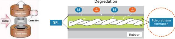
High Adhesion Retention technology (HARTech) is an advance dipping technology specially designed to protect polyester adhesion properties.
